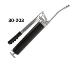
An improvement of the 30-200, this gun has a textured barrel and rubber handle grip for added ease of use. 2-way loading: 14 oz. cartridge or suction load. Includes 5-3/8" angled pipe and coupler. Added bleeder valve and locking plunger provide for easier priming. Develops up to 6,000 PSI. Delivers 1 oz./40 strokes.
